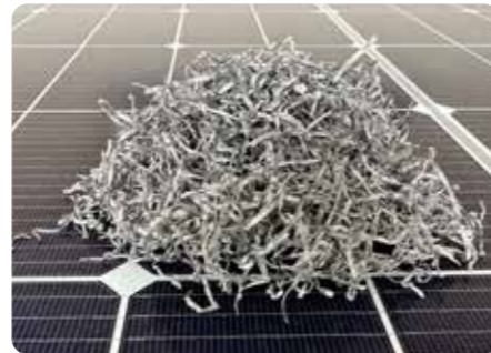
Conductors (tinned copper)
